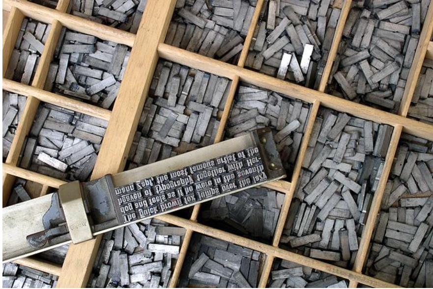
Figure 2.1: Assembling individual types. Note how the individual types are mirror-images of the letters and they must be placed from left to right.
